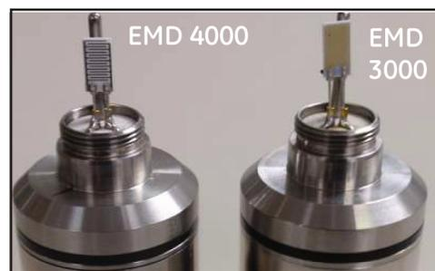
Figure 2: EMD3000 and EMD 4000 Sensors on Loggers
