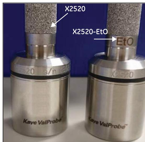
Figure 3: Loggers with and without ETO on Cap
